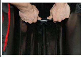
The closed **cross rib F** is placed behind the back seat.
