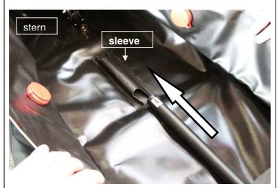
Take the **keel rod #5** (the arrow pointing towards the bow is on the rearmost position) and push it through the sleeve on the hull before clipping it to the stem element.
