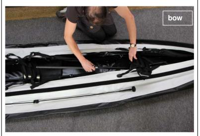
Take **keel rod #2** (with a hemispherical end) and push it with the open end through the sleeve under the front seat. Then clip it onto the stem element.
