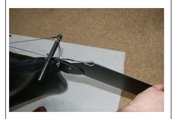
Now place the rudder onto the cavity at the stern and secure it with pin, by pushing it through from above. Secure the pin at the bottom again with the little ring.
