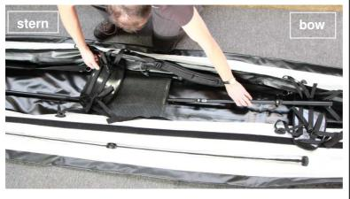
Push it **from the front** under the middle seat and clip it onto keel rod #4.
