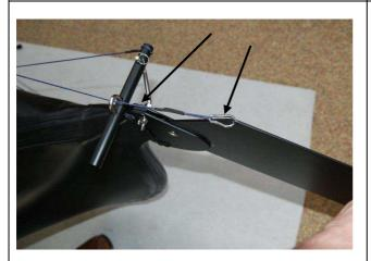
Lead the end of the pull-up rope back through pin and attach it to the rudder with the carabiner.
