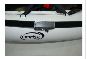
The clip for pulling up the rudder blade can be positioned as you like on the Velcro.
