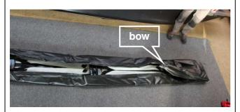
Before folding the hull, lay it out flatly. Fully drain the air from the sponsons. You can also do this with the supplied pump, since it has a suction function. Then fold the sides in the middle (lengthwise) as shown.
