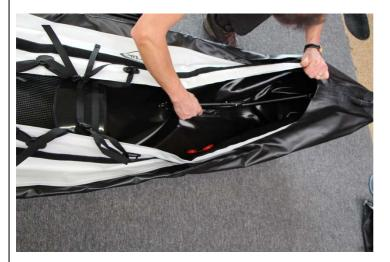
Insert the stem element as far as possible into the **stern**.
