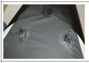
The two little tubes are the openings for the tripping lines of the rudder system, in case you want to use it.
