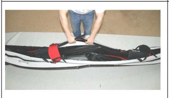
Slowly push both rods downwards into the hull. This is how the longitudinal tension is provided by pressing the frame into the hull.
