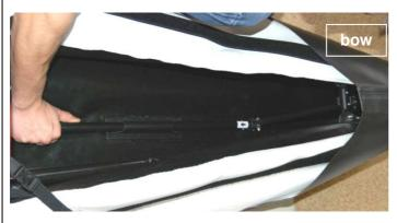
Install **keel rod #1** (two open ends and the arrow pointing towards the bow is on the forward position).
