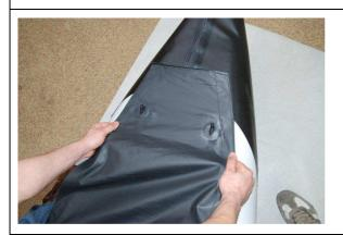
Mount the optionally available deck from the stern. Place it in such wise, the deck just covers the Velcro on the boat.
