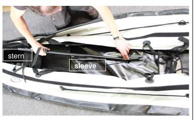
Take the **keel rod #4** (two open ends and a riveted clip) and push it through the sleeve on the hull (behind the middle seat) **towards the bow.**
