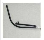
First unfold the hull and take out one of the stem elements (they are identical).
