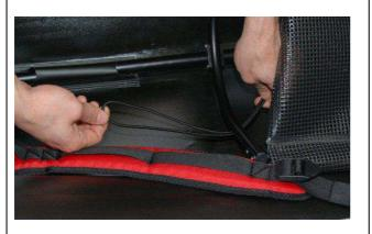
Now lead the extensions of the steering lines (with chains) from behind under the cross rib of the middle seat.
