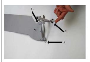
At the first assembling take the small security ring (1.) off the rudder blade.
