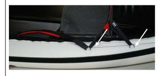
Lead the two steering lines from behind through the two D-rings, on which the back rest is attached.
