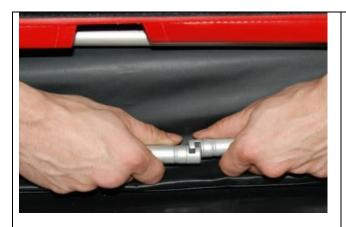
Then connect the two locks. You must align the locks exactly to another, in order to prevent jamming.
