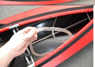
Now inflate the sponsons by using the filling tubes. These are then connected with the connecting pipe. By connecting the tubes you will provide a pressure equalization, which guarantees an ever symmetrical underwater hull.
