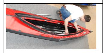
Then push the remaining two coaming rods without D-ring into the channel towards the stern and connect them to the flexible pickup elements in the stern.
