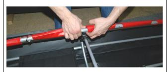
Then clip the coaming into the big top C-clips of the cross ribs.
