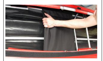
This process takes a bit more strength, when the boat is new. The seat extends a bit, so it gets easier each time. It might help to slightly press the two stringer elements inside the boat, in order to place the seat easier.
