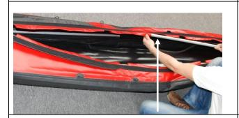
Connect one of the bent rods with D-ring with one of the short rods.
