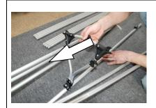
...then slide the clip onto the "counter clip" on the keel rod and slowly right it up.
