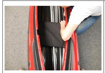
Insert the stringer elements into the seat and pull the seat backwards. Grab from behind to the front part of the seat (as on the picture below).
