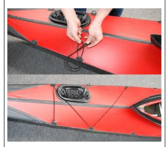
The deck lining can be installed in different ways.
