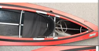
The lower straps are fixed on the cross rib behind the seat.
