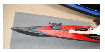
Try to orientate at the ridge bar and the reinforcement strip on the deck to insert the frame centrally. Also, a look through the hatch can help.
