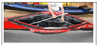
That means pulling up stern and bow ("stern over bow"). Hang keel rod #4 **under** keel rod #3 (with the riveted half-tube) and gently push the whole thing down.
