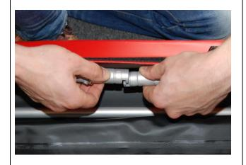
Align both locks exactly on another. Then press the rods slightly downward or upward - depending on how the connection works better.
