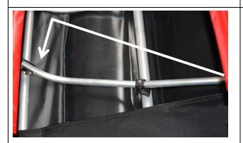
Now take the remaining half cross rib. This is to support the seat and ensures that the weight of the paddler does not press on the stringer element. It is therefore **essential to install!**
