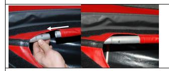
Then connect the coaming rod with the pickup element in the bow by sliding it onto it. Just pull the flexible part a bit toward you, so that there is also a straight line. Thus the connection of coaming rod is much easier.
