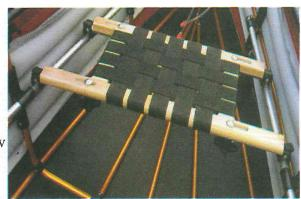
7. A revised style of the PakCanoe seat offers a wider range of adjustment. The seat's adjustment is fixed with a screw driver by tightening stainless clamps that compress the tubular sleeves under the seat to prevent any side to side movement. The clamps are secured to the seat frame. No adjustments need to be disturbed when the canoe is disassembled, and no tool is needed to reassemble the canoe.
