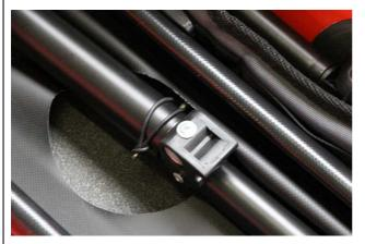
Make also sure not to twist the rods while pushing them down. If the rods are twisted, it can be difficult to re-enter the split pin in the next step.
