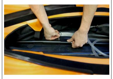
The keel rods then get connected with the split pin.
