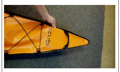
Pay attention to the sponsons not being jammed under the keel, but laying neatly to the left and the right inside the hull.
