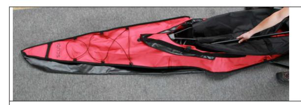
Insert the bow and the stern segments (with the attached sponsons) in the hull. (see above)
