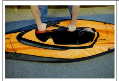
Ensure that the stem still sits neatly and symmetrical inside the hull, then slowly press the keel rods downwards into the hull.
