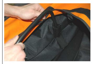
Then insert the two smaller cross ribs behind and in front of the cockpit from the top into the sleeves on the sponsons.
