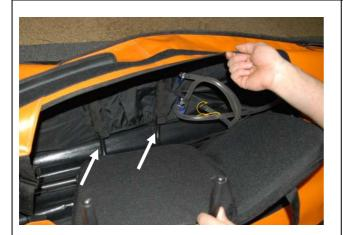
Now install the seat. Therefore, insert the cross ribs from the bottom into the sleeves at the sponsons.
