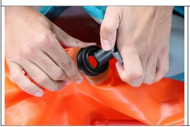
Please unfold the boat skin and unscrew the black valve. Then stick the plug of the filling bag in it, like it is shown on the image on the left.
