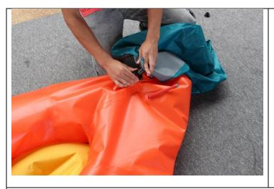
Air will be pumped in the boat with the filling bag. It needs some time getting used to in the beginning, but works very well. After 7-8 pushes the TrekRaft is so far filled, that the rest pressure can be produced with the second valve and your mouth.
