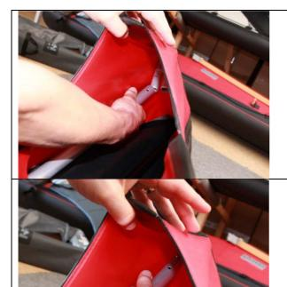
The pickup element is movable and if you stand beside the boat and pull the coaming rod back-/outwards, you'll create enough space.
