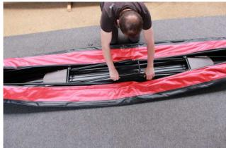
The frame is thereby "pressed" into the hull
