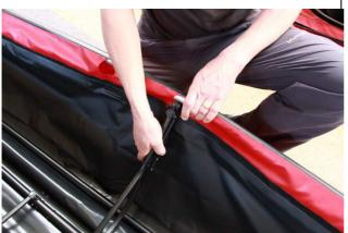
Then clip the cross rib to the coaming on both sides.
