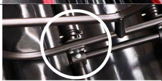
When the cross rib is placed correctly into the sockets on both parts of the keel ladder, it is firmly connected to it.
