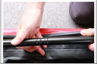
In a straight line the two locks can easily interlock.
