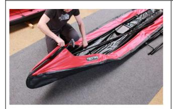
First spread out the skin. Then take the bow segment and push it into the hull.
