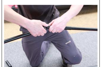
Then secure the locks with your thumb, to ensure that nor stringer element nor the lock can slide off while pressing them down afterwards.
