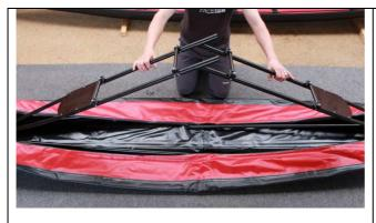
Then take the two keel ladders upwards. Place the riveted half-tube above the keel ladder with the hemispherical end. Then hang the hemispherical end under the half-tube and push the whole slowly downwards.
