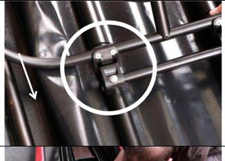
First place the cross rib diagonally, so you can slide the clip onto the "counter clip" on the keel ladder.
