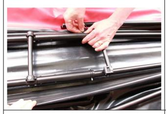
Then secure the ladders by reinserting the two split pins.
