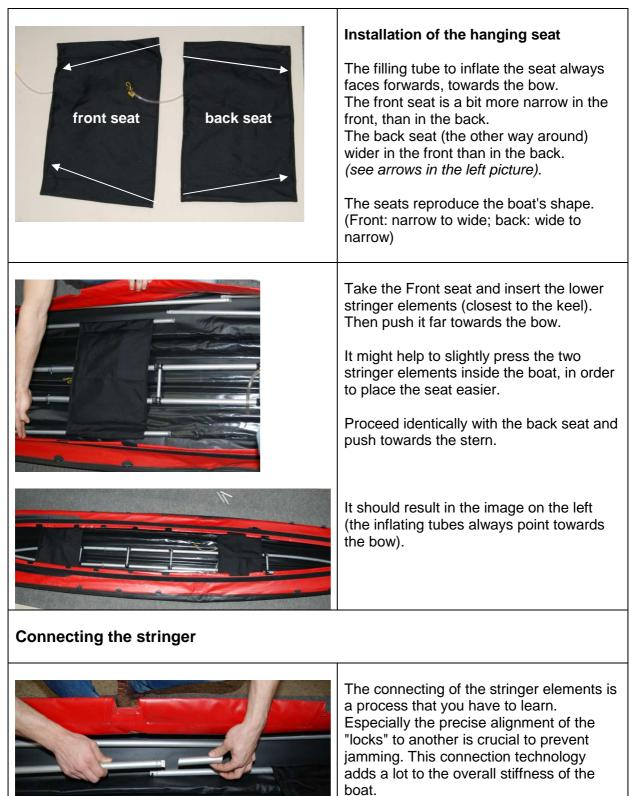
For one, you "press" the excess length, the two stringer element with lock of bow and stern have, "into the boat length" and on the other hand, this connection is stable, both on pressure and on tension. **A huge advantage on the water!**
