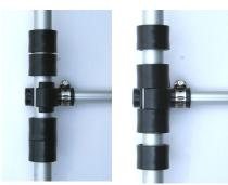
2. Determine how high you want the rail, lift the plastic rings above where you want the rail, and press the bracket into place so it clamps around the cross rib. Press the rail down so its bottom inserts into the plastic ring. Push the upper rings down onto the bracket to lock the connection.
