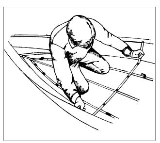
rib. Pivot the cross rib all the way so the latches snap shut. Secure the latches with the elastic bands that are installed around the latch rod. Lock the C-clips that connect the cross rib to the gunwales (see panel on locking sleeve).
