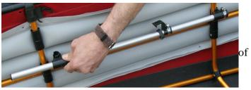
4. Install the rail on the other side of the canoe to match the placement of the rail you just installed.
